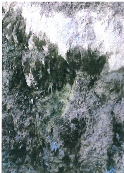
Photo 1: Groundwater seepage from bedrock outcropping at the wester perimeter of the west property, facing west, April 16, 2015.
